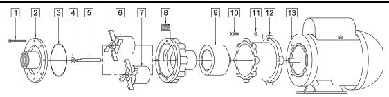
When attaching the Drive Magnet to motor shaft, position the face of the Drive Magnet 3/32 inch below the face of the Motor Bracket.
