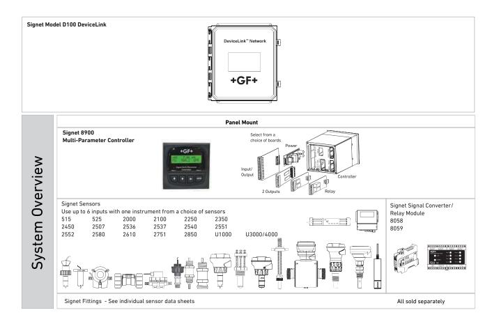
There are hundreds of system types that can be set up with the 8900. The examples below illustrate various sensors in different installation schemes. Wiring topology for point-to-point, daisy-chain, multi-drop, or a combination of these are listed in each example. Digital sensor outputs allow for long cable runs with high noise immunity. See Wiring section for allowable cable lengths.
