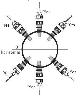
When mounting in standard threaded fittings the electrode must be mounted horizontally to 60 degrees below horizontal position only.
