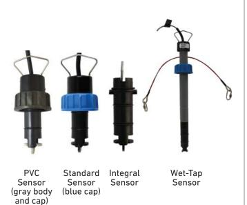
Simple to install with time-honored reliable performance, Signet 2536 Rotor-X Paddlewheel Flow Sensors are highly repeatable, rugged sensors that offer exceptional value with little or no maintenance. The Model 2536 has a process-ready open collector signal with a wide dynamic flow range of 0.1 to 6 m/s (0.3 to 20 ft/s). The sensor measures liquid flow rates in full pipes and can be used in low pressure systems.
