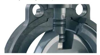
The shaft, disc and face seals all operate independently from one another. This eliminates issues common to booted style centric valves such as crimping, where the compression of the valve between two flanges causes the boot to ripple. This can lead to increased operating torque and wear, ultimately reducing the useful life of the valve.
