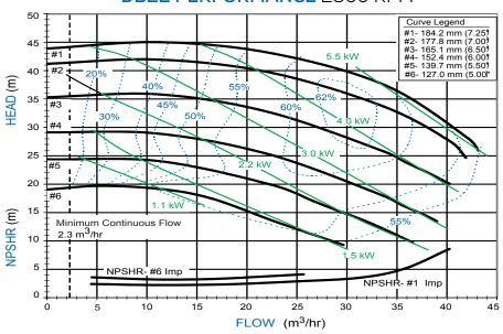
Notes: Performance curves above are based on closed impellers. Contact the factory for performance based on open impellers.
