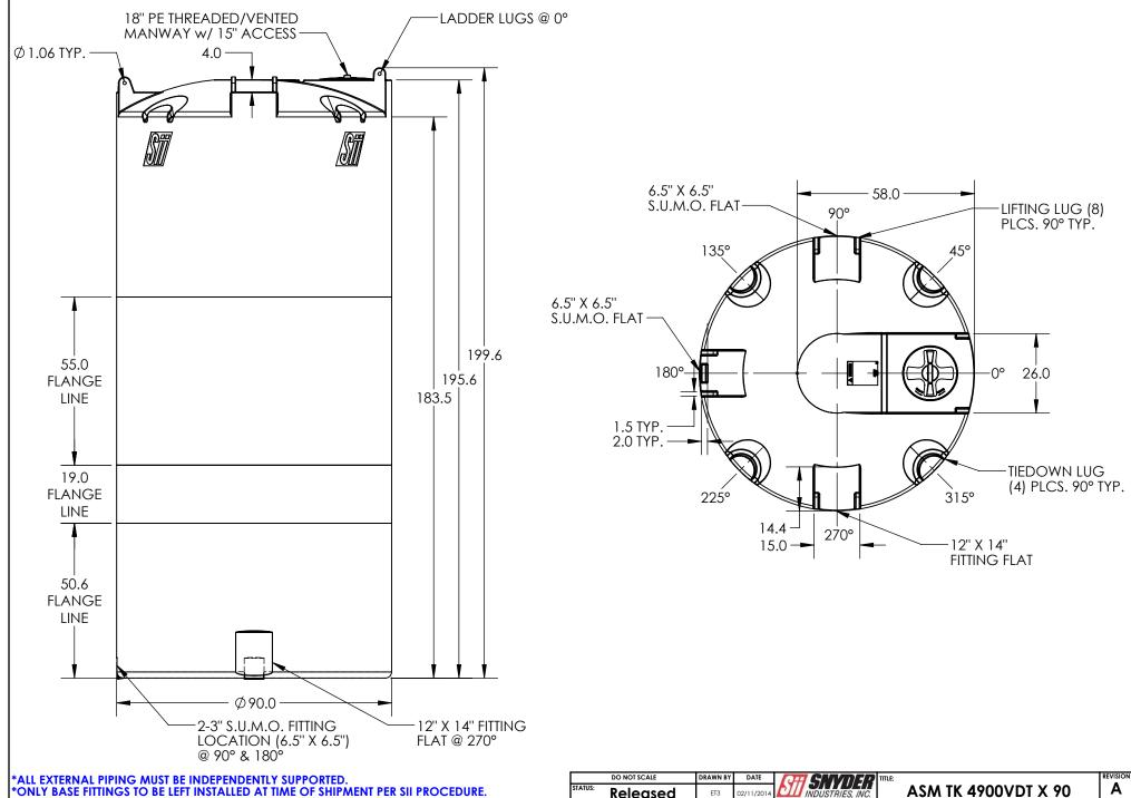
Available on-line at http://www.snyderindustriestanks.com/Technical ALL DIMENSIONS ARE IN INCHES, NOMINAL, & SUBJECT TO CHANGE WITHOUT NOTICE. ALL DIMENSIONS ON ROTATIONAL MOLDED PARTS ARE SUBJECT TO A ± 3% TOLERANCE.
