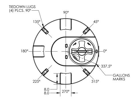
NOTES: GALLONAGE MARKS MAY BE REMOVED FOR FITTING PLACEMENT AS NEEDED.
