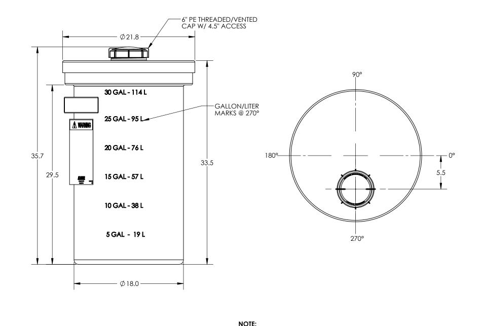
\*ALL EXTERNAL PIPING MUST BE INDEPENDENTLY SUPPORTED. \*ONLY BASE FITTINGS TO BE LEFT INSTALLED AT TIME OF SHIPMENT PER SII PROCEDURE. \*Consult Snyder's Guidelines for Use and Installation prior to delivery. Available on-line at http://www.snyderindustriestanks.com/Technical
